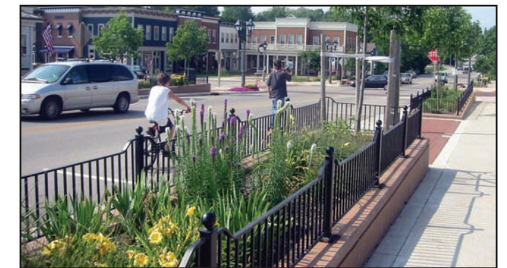
Planters and landscaping separate pedestrian space from parking, bike and drive lanes.
