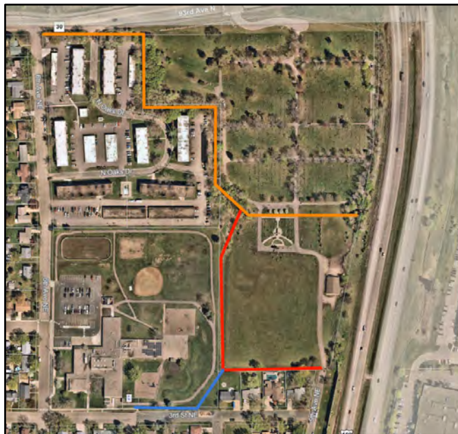
Figure 1. Extents of the proposed ditch maintenance project (orange), tributary ditch (red), potential future storm sewer extension (blue).
